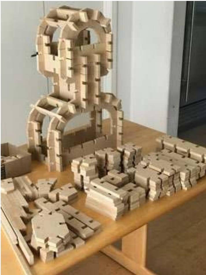
Using only a table saw and a miter saw, you can make your own set of interlocking wooden toy blocks.
